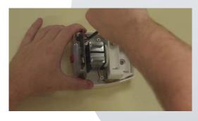
Fit the supplied batteries (2 x "C" cells). Note, the correct orientation is marked in the battery compartment. The motor will turn for around five seconds.
