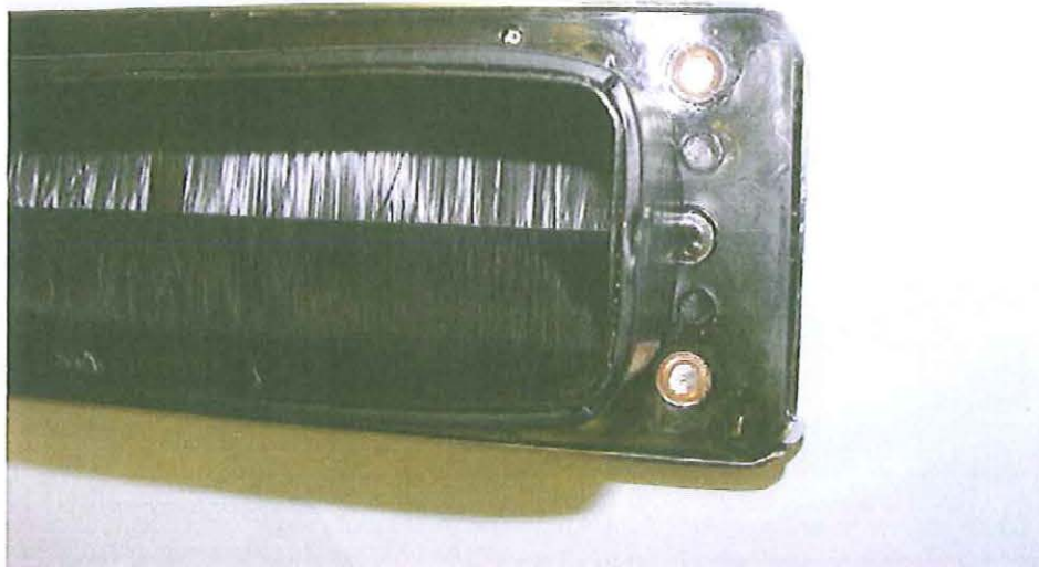
Photo 4: Detail of brush and intumescent material around synthetic middle section
